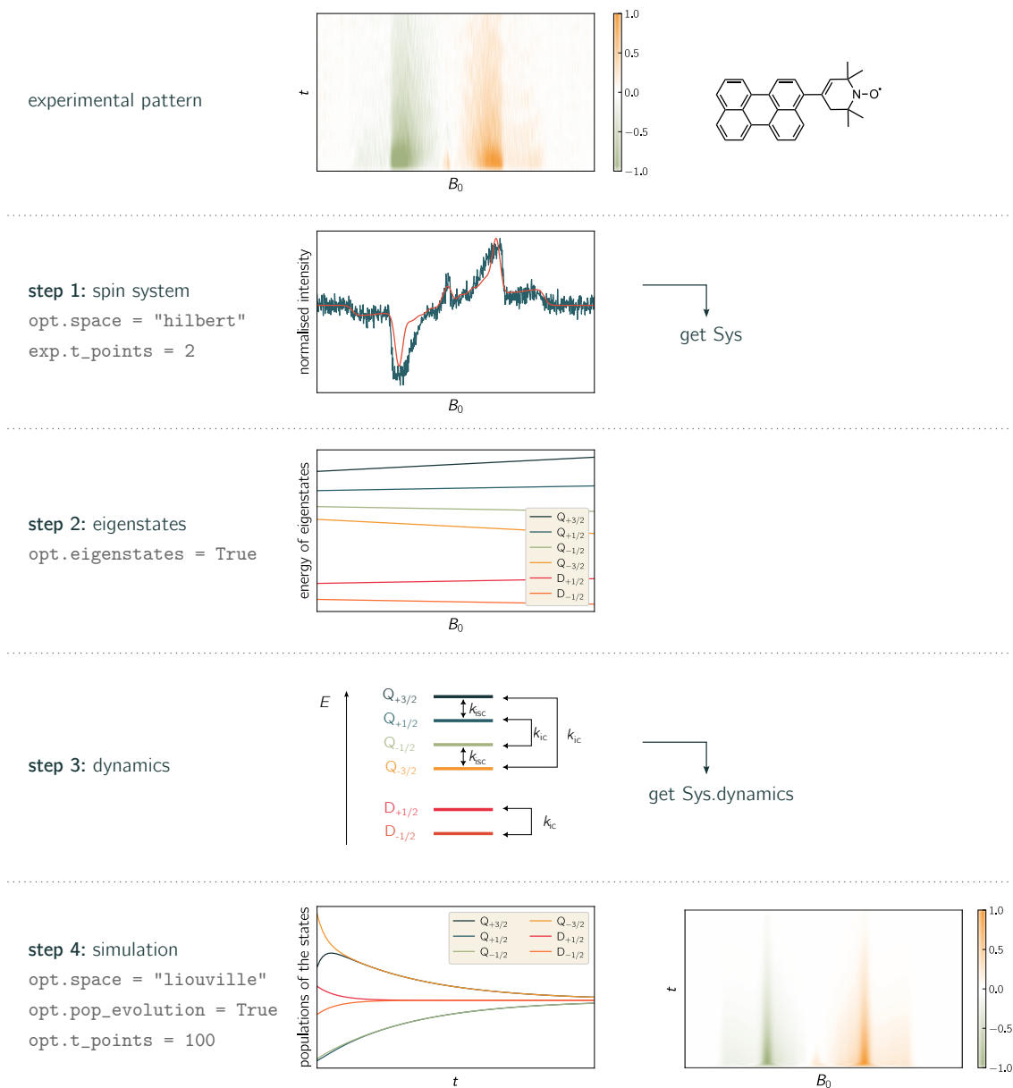
Figure 4: From an experimental spectrum to a teacups simulation. The simulation of a time-resolved EPR spectrum requires four steps which are illustrated here on the example of a photoexcited perylene–nitroxide molecule forming a triplet–doublet pair. 86 The spin system parameters are determined by a quick Hilbert-space simulation of the EPR spectrum at early times after photoexcitation. The doublet and quartet eigenstates are plotted. Two rate constants, for intersystem crossing (isc) and internal conversion (ic), were chosen here to describe relaxation processes between the states. The whole spectrum and the evolution of the populations is finally plotted. Important simulation options are indicated in grey and the resulting plots are shown for each step. For a better illustration of the workflow, any ticks and tick labels were omitted in the plots of the experimental data. Experimental details and simulation parameters are provided in the SI (Section 3 and 4).
